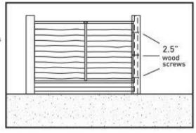
If the first post is in open ground it will again need to be upright and perpendicular to the ground in both vertical planes and facing accurately in the correct direction. Mount in concrete as detailed below then attach to the first fence panel using 2.5" wood screws.
