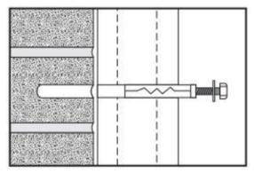
less than two in total. Drill the holes in the post first and allow only a small clearance over the shank diameter of the anchor bolt. Offer the post to the wall ensuring it is level in both vertical planes and aligned correctly (using a spirit level and engineers square). If necessary use packing between the post and the wall. Bolt the post firmly into position.
