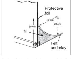
on of the bottom frame with the SP wall with a protective liner. Such a liner will stop any material that could enter the grove of the frame and damage the structure of the SP. What can be used as the liner is any plastic foil forming a strip of approx. 40 cm.
