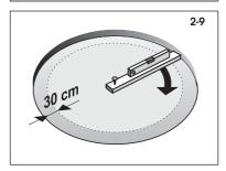
**Remember:** A strip of 30 cm of width around the circle must be in perfect level, see fig. 2-9. The bottom edge of the pool's side must be in level and must not lie on top of a depression. Pay attention to make sure the area is absolutely plane and in perfect level.
